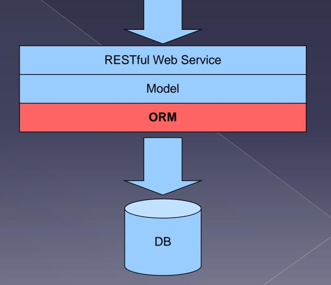
Store and load data from an RDBMS into an Object Oriented Data Model
